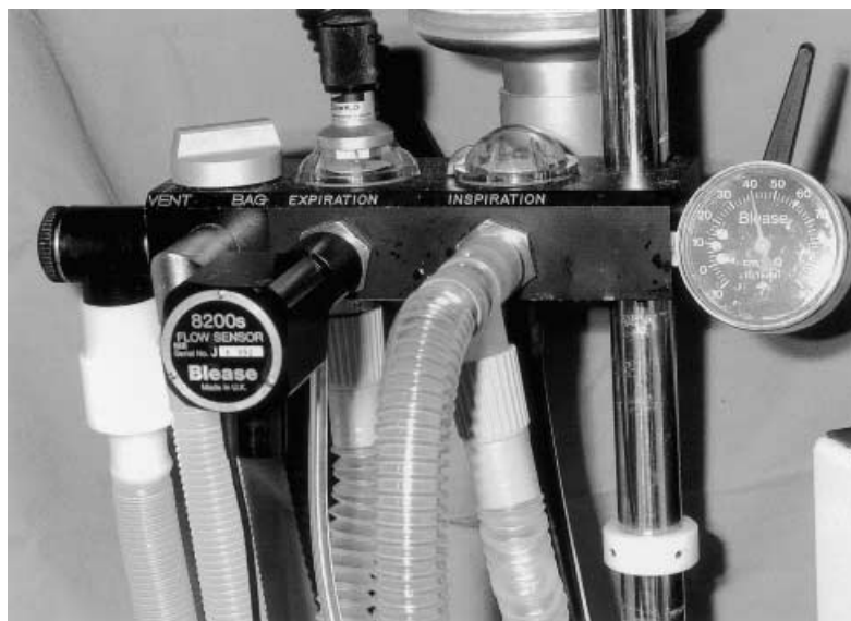
Figure 6 Expiratory limb of the breathing system misconnected to the patient safety valve of the Scandia absorber circuit block resulting in expiratory obstruction.
